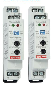
These single thermostats are for temperature monitoring and regulation in control panels, heating systems, cooling systems, liquids, radiators, motors, devices, open spaces, etc. The Thermtec-SL60 has a temperature range of 0°C to 60°C and the Thermtec-SL45 has a temperature range of -15°C to 45°C.
